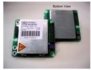
It sends an energizing signal to the transponder, modulates the RF signal to send data to the transponder, receives the identification signal and processes it for digital decoding. The small size and low supply voltage make the Mini RF Module well suited for portable read/ write units.
